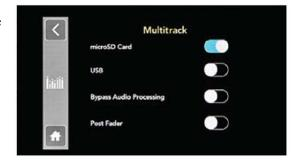
You might notice that, after recording your multi track podcast to a microSD Card and listening back to it on your computer, all channels are the same volume, with none of the mixing you did before or during recording carrying over to your multi track files. This is because in its default mode, the RØDECaster Pro will always record in **pre-fader**.
